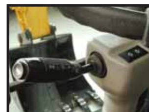
Tiltable steering wheel with several functions; wiper control, indicator, horn, and headlight
